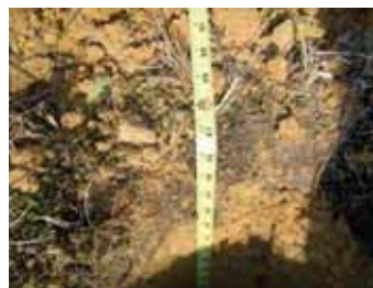
Depth of test pit was approximately 4 feet
